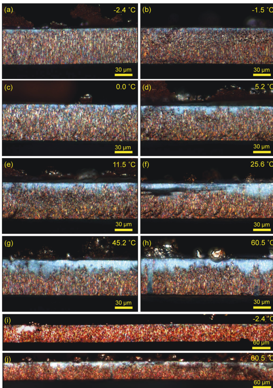
Figure 3 Optical microscope images of the cross sections of the AAO template with Cu nanowires. These are grown at various deposition temperatures: (a) -2.4°C; (b) -1.5°C; (c) 0.0°C; (d) 5.2°C; (e) 11.5°C; (f) 25.6°C; (g) 45.2°C; (h) 60.5°C. (i) and (j) show large-scale view of the cross sections at -2.4°C and 60.5°C, respectively. Yellow arrows indicate empty pores.
